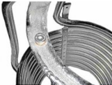
Ref - coil jet ring clean and drain position
