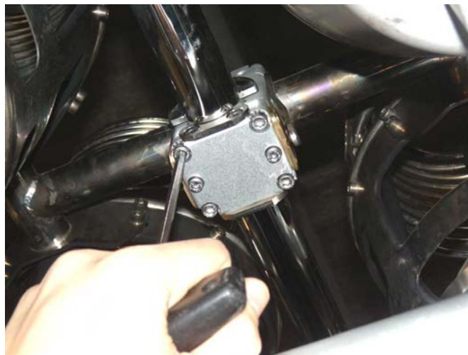
Figure 3 – Unscrewing the Gimbal Bottom Cap
