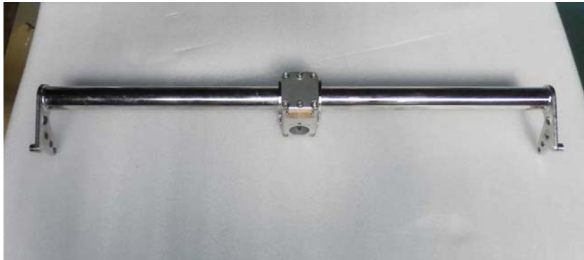
Figure 2 – Triple Burner support tube with gimbal block assembled
